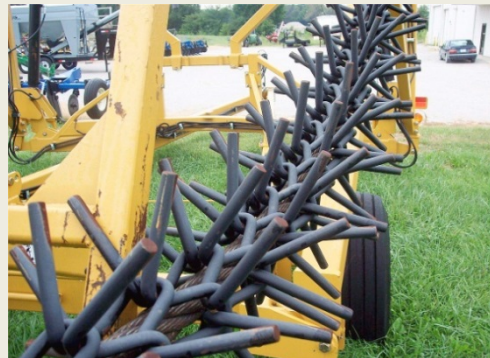
Phillips 4500 rotary harrow showing rotating tines and interlocking offset arrangement. (Photo from Kelley Manufacturing Co.)
